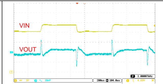
图 2 Line Transient ( V_{IN} =from 4.3V to 5V to 4.3V, I_{OUT} =300mA)
