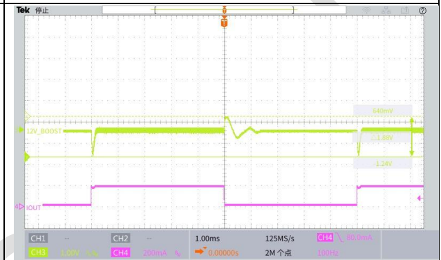
12V Load Transient, SCAP=2.5V, IOU=20mA- 200mA, 0.3A/us
