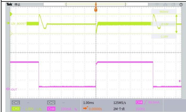
12V Load Transient, SCAP=2.5V, IOU=30mA-300mA, 0.3A/us
