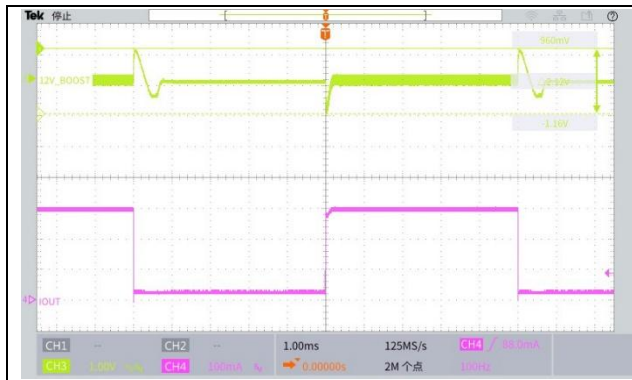
12V Load Transient, SCAP=2.5V, IOUT=30mA- 300mA, 0.3A/us
