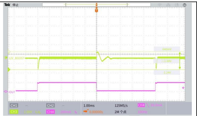
12V Load Transient, SCAP=2.5V, IOUT=20mA- 200mA, 0.3A/us
